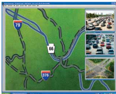
In Picture-in-Picture Mode, you can view the full screen display on one video source along with smaller images from the three other video sources.
