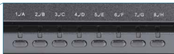
KVM switch selection buttons on the monitor bezel (above) enable switching between servers with only the LCD panel open.
